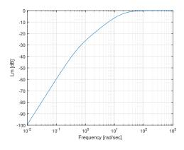
Fig. 6. Log-magnitude plot of M (vide small-gain theorem)
