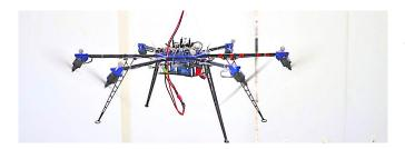
Fig. 1. The considered hexarotor with tilted propellers (Tilt-Hex).
