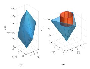
Fig. 2. (a) Feasible force set of the platform in Fig. 1 at hover. (b) The same feasible force set with cross section at the gravity plane. The figure also shows the BLF cylinder for the platform applying a lift force  $\pm 20\%$  of the gravity opposing lift.
