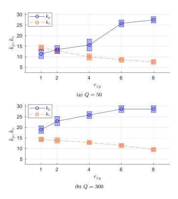
Fig. 4. Optimized gains  $(k_p, k_v)$  of the position controller versus  $\overline{f_{xy}}$  for two values of the weighting ratio Q. For each optimized gains, we show the average value and the standard deviation bar computed from three repetitions of each experiment.
