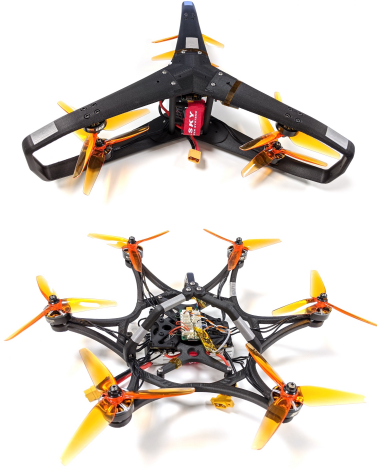
Fig. 3: The Y-shaped (top) and Star-shaped (bottom) hexarotor platforms built in-house for the fair comparison.
