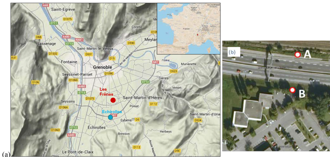
Figure 1. (a) Location of sampling sites in the Grenoble Alpes conurbation: the roadside site (Echirolles) and the urban background site (Les Frênes). (b) Echirolles sampling site: sampling and measurement devices are around the B point; the traffic electromagnetic loop monitoring is beneath the road (on the AB line), on the left; and the cameras linked to automatic license plate recognition code are located on overhead gantries.
