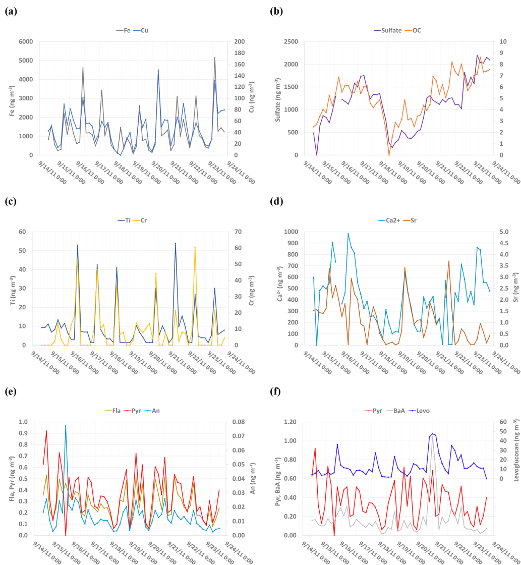
Figure 3. The 4 h concentrations measured at the traffic site: (a) iron and copper; (b) sulfate and organic carbon; (c) chromium and titanium; (d) calcium and strontium; (e) fluoranthene, pyrene and anthracene; and (f) pyrene, benzo(a)anthracene and levoglucosan.
