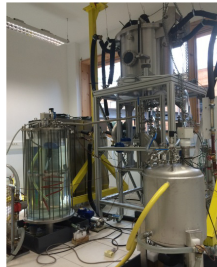
Fig. 6: Picture of the PROSSIS2 prototype: in front, the water storage tank, in glass: the solution storage tank, above: the reactor
