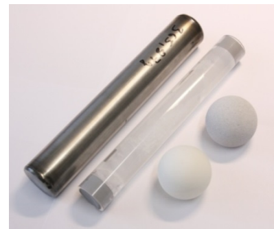
Fig. 22: Macroscopic encapsulated PCM for mobile latent thermal energy storage of University of Bayreuth
