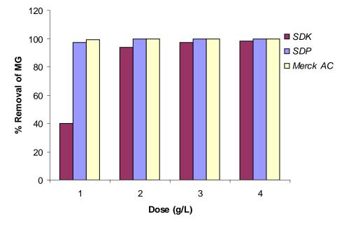
Fig. 1 Dose effect of MG adsorption.
