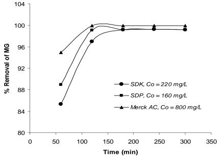
Fig. 1 Contact time effect of MG adsorption Example 1
