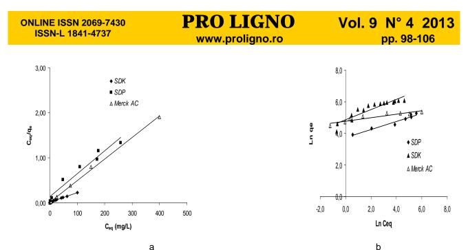
Fig. 2 Linearized adsorption isotherm of MG (pH=6, dose = 8g/L, t = 2h) a - by Langmuir; b - by Freundlich.
