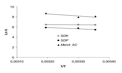
Fig. 4 Fig. 4 Plot of In  $K_c$  vs 1/T for thermodynamic parameters estimation.
